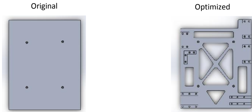
Figure 10: Initial & Optimized Base Plate [10]
