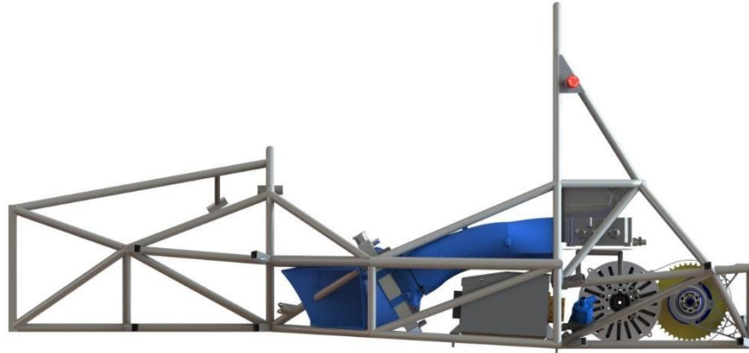
Figure 14: Ductwork design two
