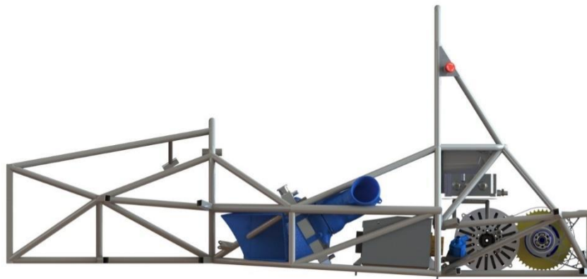
Figure 13: Ductwork design one
