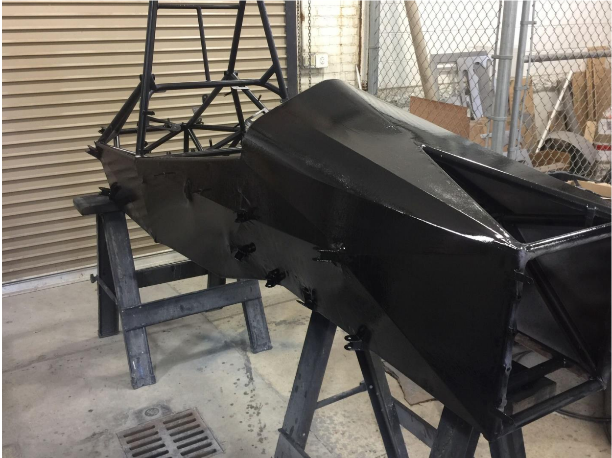
Complete Painted Frame with Aircraft Fabric Coating
