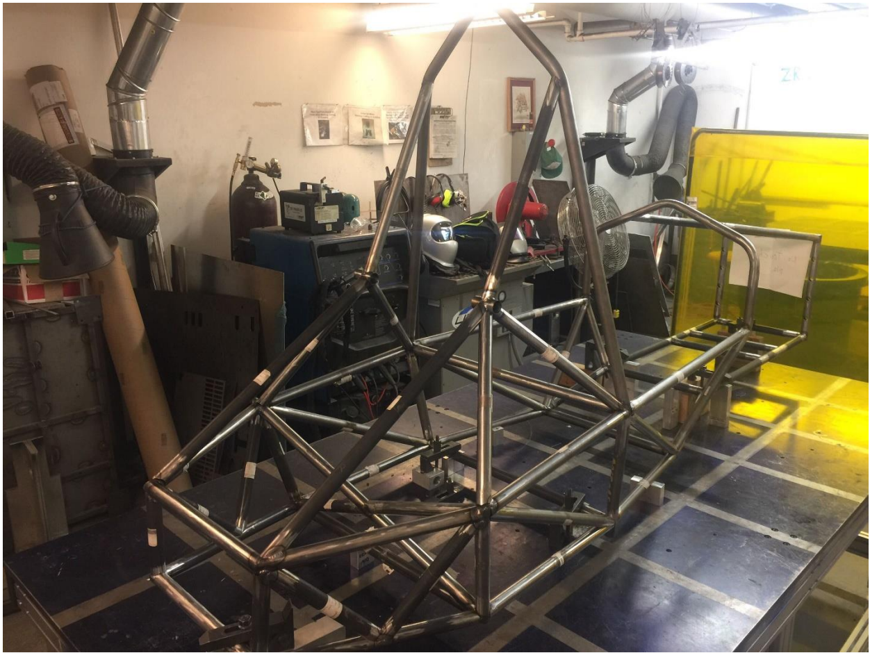
Rear of Frame after welding in Super node and Main Hoop Braces and Supports
