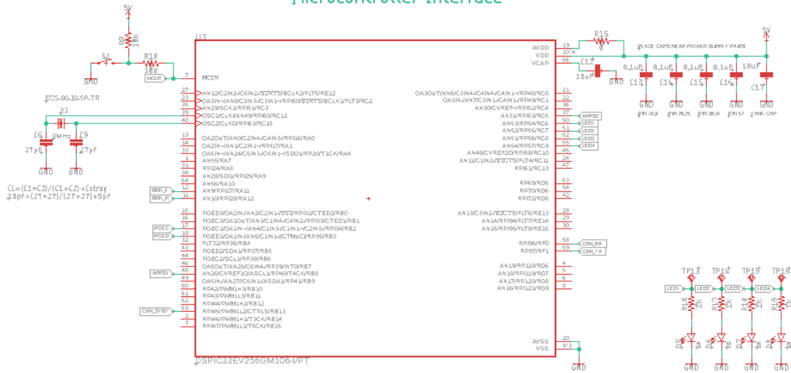
Figure 10: A/CAN PCB Schematic – Microcontroller
