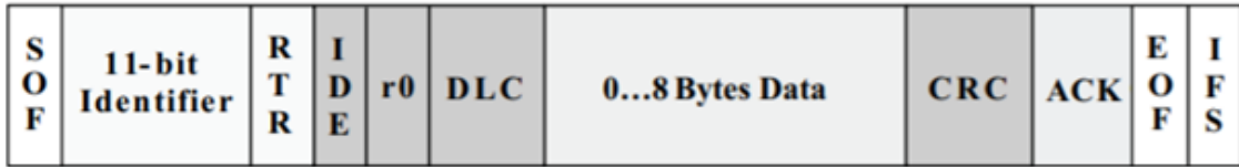
Figure 2: Standard CAN Message, (Corrigan, S)
