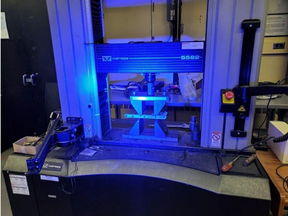
Figure 15: setup of the prototype pedal in the Instron machine.
