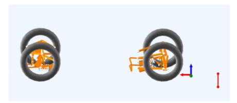
Figure 12: ZR19's kinematic pitch center as seen in its most rearward position during a typical acceleration.
