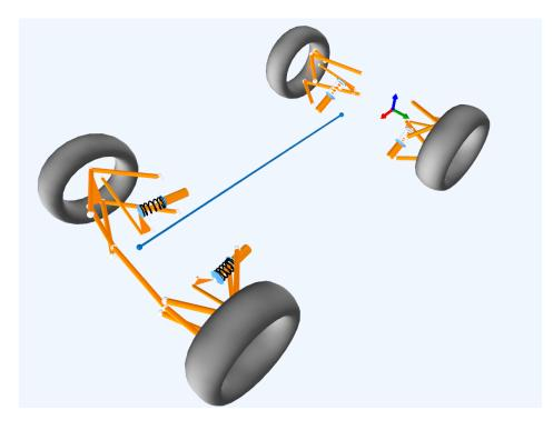
Figure 20: Roll Center of ZRE-20 at -2 Degrees of Roll
