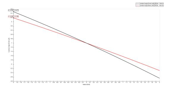
Figure 25: Camber Angle of ZRE-21 under Roll
