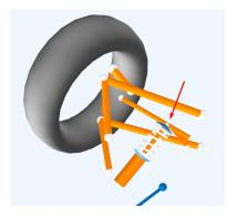
Figure 23: Damper hitting Pull-Rod
