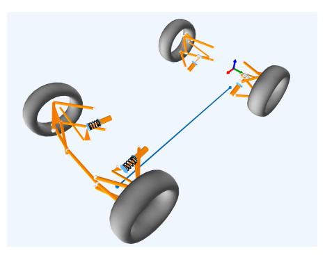
Figure 21: Roll Center of ZRE-20 at 2 Degrees of Roll
