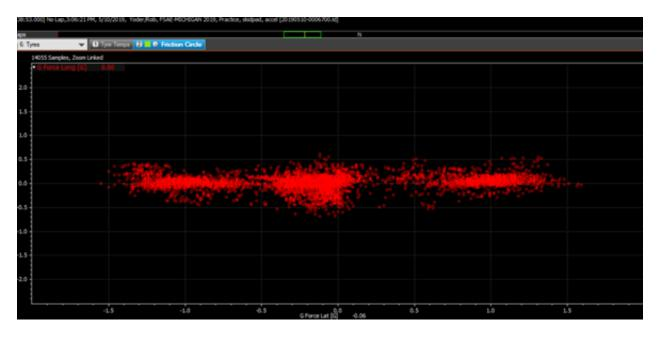
**Figure 8:** Friction Circle for ZR19 from the skidpad event at Formula SAE Michigan 2019. The best time in this skidpad event was a 5.36 second time, or 33rd out of 109 teams at the event.
