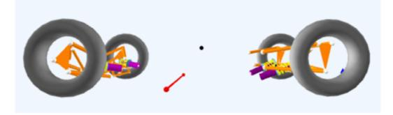
Figure 17: ZR20's kinematic pitch center in its frontward-most position during a typical heavy braking scenario.
