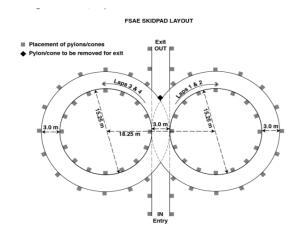
Figure 6: Official layout, including dimensions and cone spacing, of a Formula SAE/Formula Student Skidpad Layout
