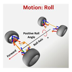
Figure 10: A generalized look at the roll axis and roll behavior of a vehicle in regards to dynamic driving scenarios (Optimum)
