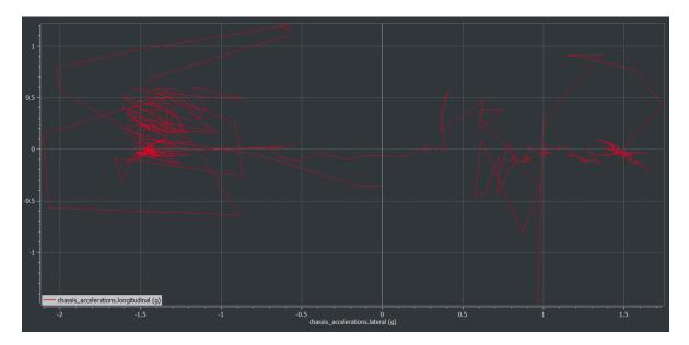
**Figure 18:** Friction Circle in VI-grade utilizing ZR20's suspension points on a skidpad run. The model was capable of running a 4.93 second skidpad lap time.
