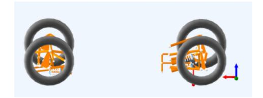
**Figure 13:** ZR19's kinematic pitch center in its center position; this can be assumed to be the pitch center during a steady state driving scenario.
