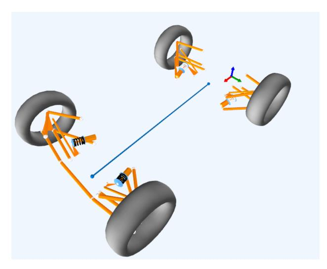
Figure 27: Roll Center of ZRE-21 at -2 Degrees of Roll
