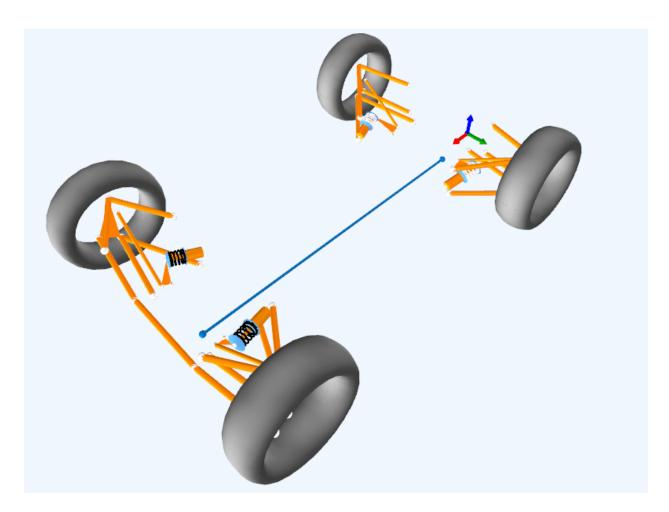
Figure 28: Roll Center of ZRE-21 at 2 Degrees of Roll
