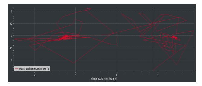
**Figure 7:** Friction Circle in VI-grade utilizing ZR19's suspension points on a skidpad run. The model was capable of running a 5.21 second skidpad lap time.
