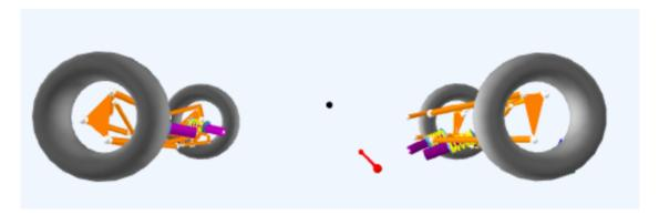
**Figure 16:** ZR20's kinematic pitch center in its center position; this can be assumed to be the pitch center during a steady state driving scenario.
