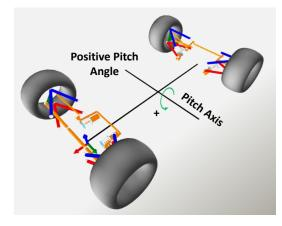
Figure 11: A generalized look at the pitch axis and pitch behavior of a vehicle in regards to dynamic driving scenarios.
