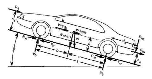
Figure 29: Arbitrary forces acting on a Vehicle (Gillespie 11)
